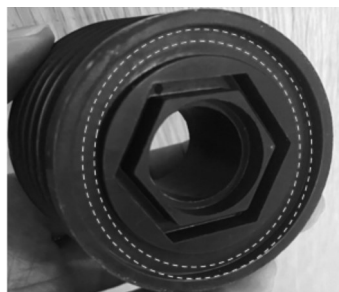
图6 套管密封不良导致电容器受潮缺陷 Fig. 6 Damp defect of capacitors due to weak sealing of bushing
