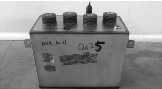
图18 直流叠加工频交流加速老化试验后试品外观 Fig. 18 Appearance of the test sample after DC stacking and frequency-modulated AC accelerated aging test
