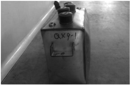
图17 直流叠加工频交流加速老化试验后试品鼓肚 Fig. 17 Test sample bulging after DC stacking and frequency-modulated AC accelerated aging test
