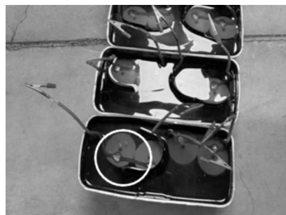
图7 元件试品不封盖导致电容器受潮缺陷 Fig. 7 Damp defect of capacitors due to uncovering of the component sample
