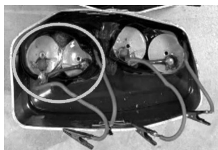
图5 喷金端部暴露缺陷 Fig. 5 Exposed defect at the metallization end
